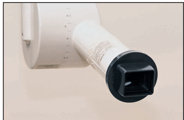
Figure 1. A snap-on rectangular collimator inserted in a circular collimator.
